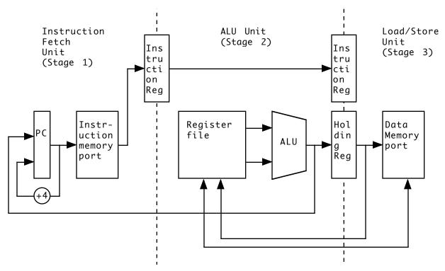
a. There are three functional units - an instruction fetch unit, an ALU, and a load/store unit - corresponding to the three stages of
