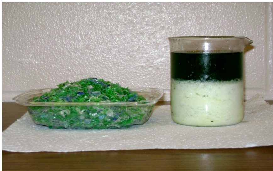
Figure 2 - Shows separation of dyes from PET that has been depolymerized
