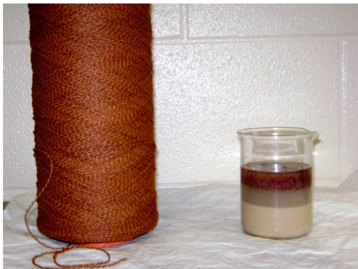
Figure 4-b - Depolymerized nylon 6 from carpet yarn
