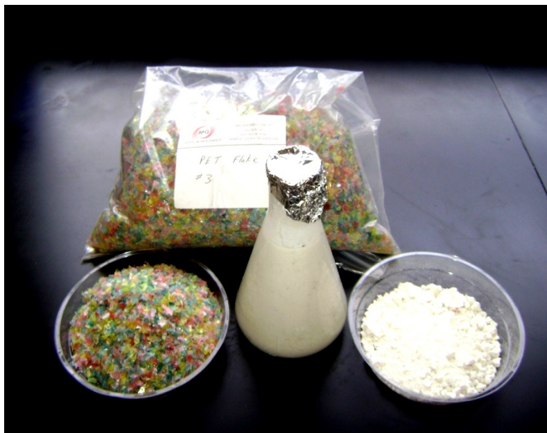
Figure 3 – Shows the separation of dyes from multiple colored PET flakes.
