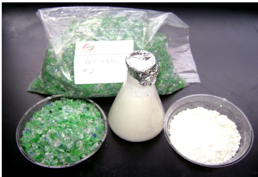
Figure 1 – Shows a) PET prior to depolymerization, b) after DP and phase 1 separation with green dye c) dried PET product.
